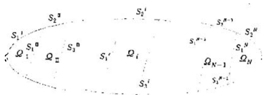
Fig. 1 Divided domains of the acoustic structure
