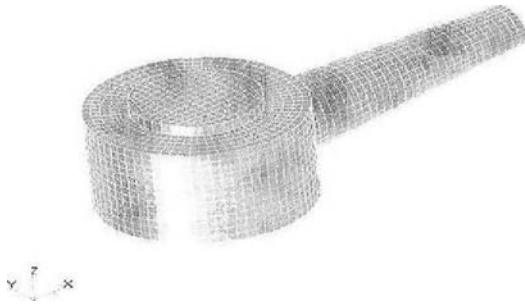
Fig. 2 Boundary element model of the air suction silencer
